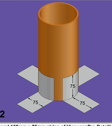
Bond 150mm x 75mm strips of VisqueenPro Detailing Strip as shown. Strips to be bonded 75mm onto pipe and 75mm onto membrane.
