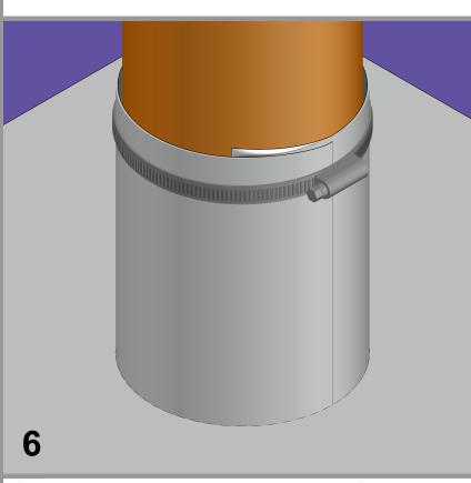
Secure upstand collar with a mechanical fastening.
