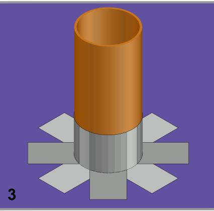
Bond additional strips overlapping previous strips by minimum 25mm.
